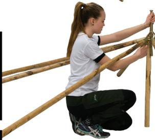
3. Rotate the main poles so that the drilled hole is horizontal.
