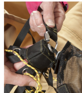
Attach the accessory connector to the top, around the band which holds the cap and ventilator cap together.
